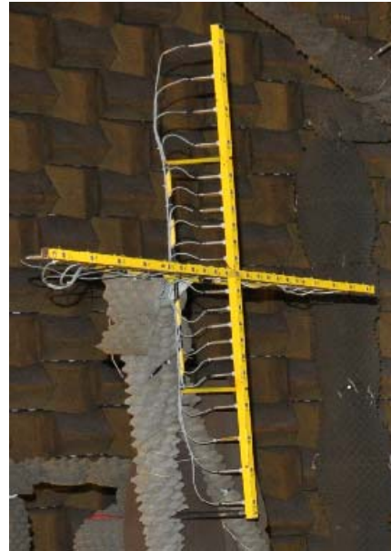
Flyover 41-microphone antenna
